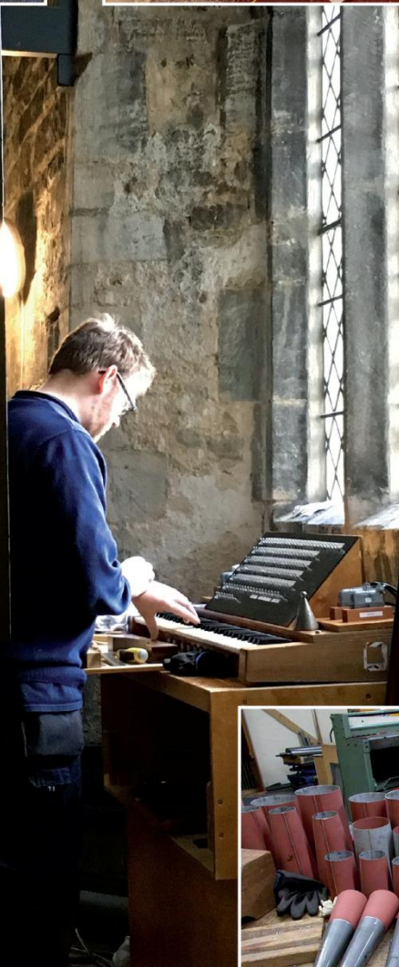
Main picture: regulating the Pedal pipework in the triforium Top left: Great 8ft Posaune hoods Top right: Pedal Open Diapason lengthening Bottom right: Swell 8ft Horn extensions
